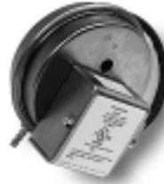
Used to automatically activate P-Series Duct Booster when dryer is in operation. DR-10 is a positive pressure sensing switch that recognizes dryer operation and activates the booster fan from an independent electrical circuit. Eliminates connections through the dryer circuit as well as manual systems which require attention of the operator.
