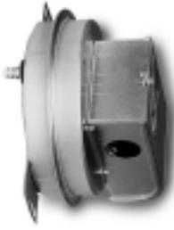
The Tjernlund Duct Airstat is used to automatically activate Duct Booster fans by sensing positive pressure in a forced air heating and/or cooling system. The single pole, single throw, snap-acting switch is activated by a diaphragm with a factory installed sampling probe inserted directly into the duct or plenum.
