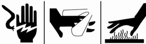
**WARNING!** Electric shock hazard, rotating fan, hot surface hazards. Unplug unit before opening cover for cleaning or servicing.
